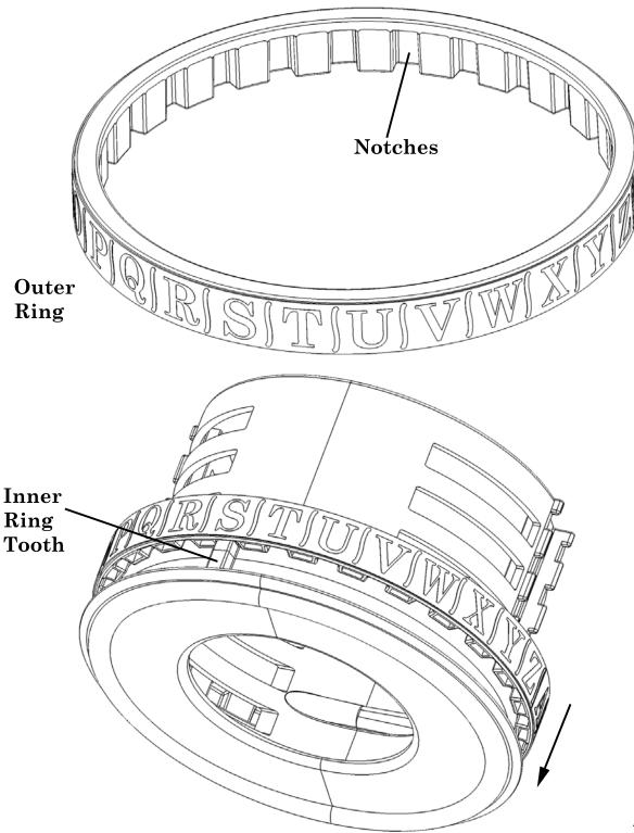
5. Replace the remaining rings, aligning "E", "N", "I", and "V" with the teeth of the inner rings. The new code word "VINES" should be facing you with the spelling from top to bottom.
