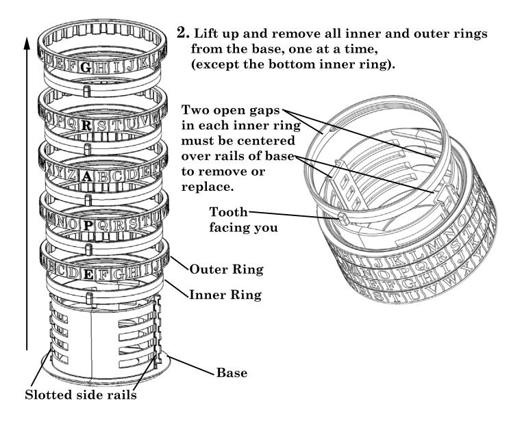
3. With rings removed, (except for bottom inner ring) place base in front of you as shown - slotted side rails positioned left and right, tooth facing you.
